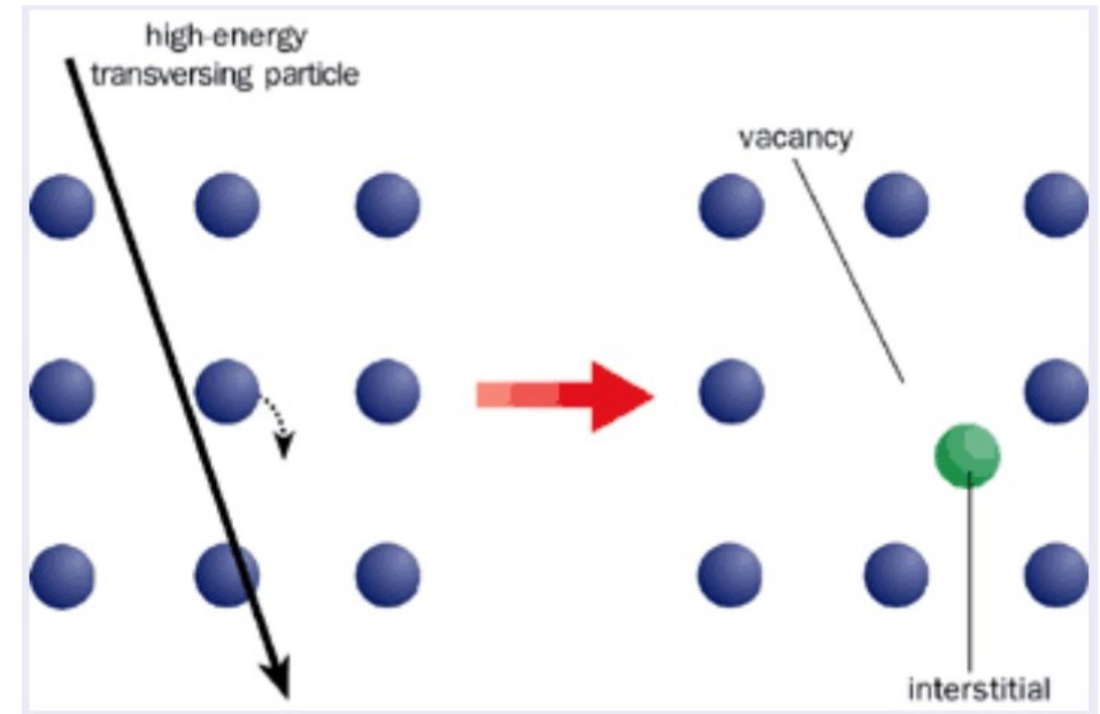
*Strategy: Irradiate CCD with neutron source to create nuclear recoils and search for new defects at "high" temp (e.g., 225K).*
