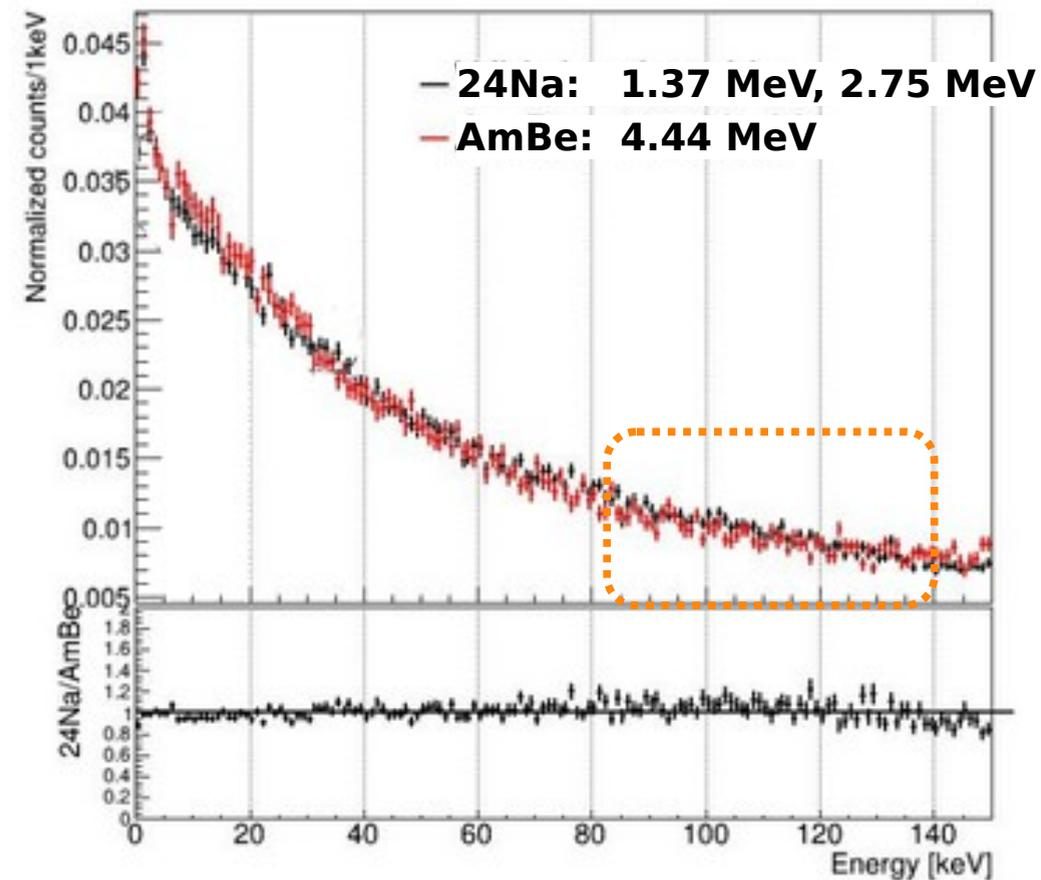
Scale  $^{24}\text{Na}$  to NR-subtracted AmBe spectrum in “high-energy” range...
